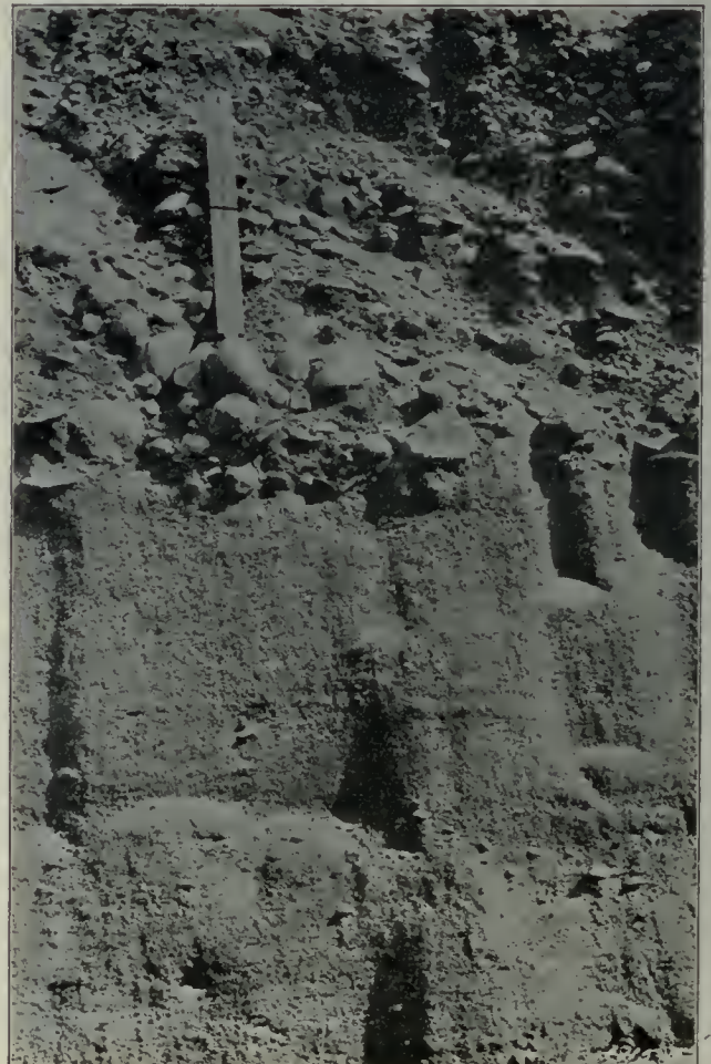
Inferior Gravel—Irregular and sandy. Note foot-rule.
